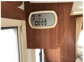
On your left as you walk in the cabin door you will find this control panel. The left button indicates level of water and electrical charge.
