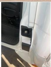
To access the diesel filler cap, the driver's door must be opened, then lift the flap to the filler cap. The ignition key is required to open the filler cap.
