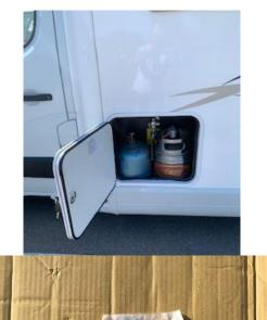
On the left side of the van, is the gas locker. The locker has room for two gas bottles. In the picture you see a French gas bottle on the left and a Spanish bottle on the right. We do not recommend putting two French gas bottles in the locker as it is a very tight fit. The Spanish bottle has a different fitting and an adaptor is attached to the bottle. The Spanish bottle can be refilled in Norway & Sweden and swapped in Spain & Portugal.
