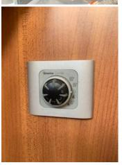
Inside the van, at the foot of the bed, you will see this knob for the hot water system. If you turn the knob so the pointer is up from the off position, the water heater will heat the water to the temperature selected. If you turn the knob so the pointer is down from the off position, the water heater will come on along with a fan to blow hot air into the camper. The heater is very efficient. Please note, the hot water will heat faster without the fan heater on.
