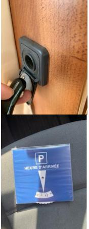
Lower the flap to find a 12v charging point that can be used while stationary. The other 12v charging points in the van are in the dash board and only work while the ignition is on.
