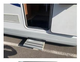
Here you can see the step is out. Remember to always retract the step before driving anywhere. It is important to double check that the step is in. The step is not automatic, you must press the button to retract it. There is no alarm on the step to warn you that it is out. There used to be an alarm, but these alarms are notorious for not working properly. It is better to be in the habit of checking every time.
