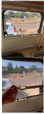
Here you can see the vents for the fridge. Behind the vents you will find an insect screen. It is important to keep the screen clean. In very hot weather, say more than 30 degrees, you may wish to remove the insect screens to allow better air-flow for the fridge. It is a good idea to park the van so that the fridge vents are in the shade, or use the awning to shade the fridge vents in the height of summer.
