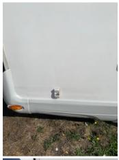
Alternatively, the awning legs may be secured to the attachments on the side of the van. This photo shows the attachment towards the rear of the van.
