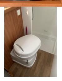
The top portion of the toilet can swivel to the position you find most comfortable. This view shows it pointing towards the shower cubicle.
