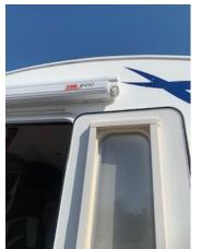
To open the awning, place the long handle into the eye on the right-hand side of the awning and turn slowly.
