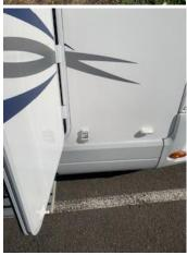
When securing to the side of the van, the other awning leg attachment is behind the door, so it can only be used this way with the door half open.
