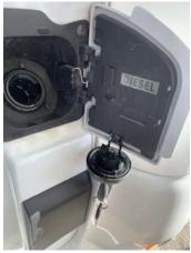
You will find a small hook on the inside of the flap, to hang the filler cap during filling
