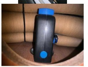
This is the reset button for the hot water system. If the outside temperature drops below 4 degrees Celsius, a safety valve will empty the hot water boiler and disable the hot water heating function in the camper. Then you must use this reset button to enable the water heater to function again.
