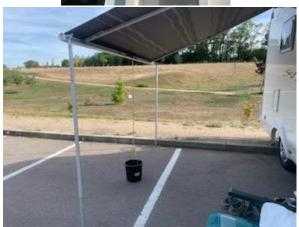
Once the awning is out and legs down, it is important to secure the awning. A gust of wind can cause major damage to the awning and the van if the awning is not secured. In this photo you can see a bucket of water has been used to anchor the awning safely. There are anchor pegs that can be hammered through eyes in the feet of the legs if you are on suitable ground for pegging.
